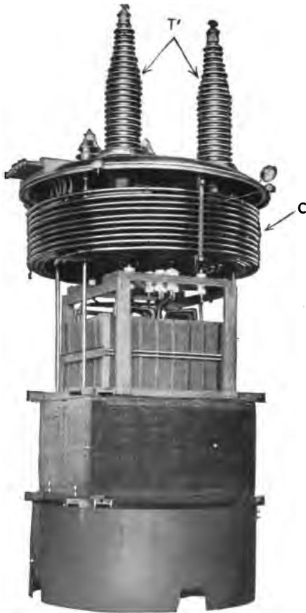
FIG. 80. Interior of an oil-insulated water-cooled transformer, showing the copper cooling coils, C. These coils carry water which cools the oil. General Electric Co.
